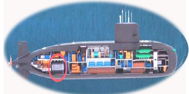
Illustration of the Chinese S-26 submarine, an oxygen tank for a Stirling cycle AIP system circled in red. China Shipbuilding Corporation Graphic
