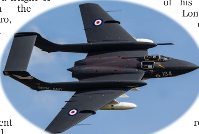
A Sea Vixen showing the pilot's offset cockpit and the observer's 'coalhole'
