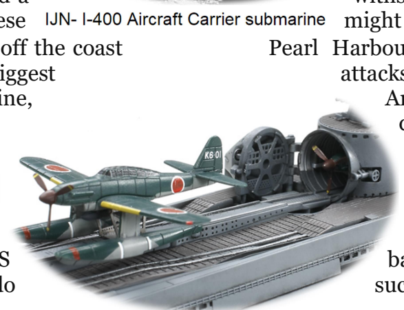
Model of one aircraft on launch rails with 2nd one ready to be rolled out
