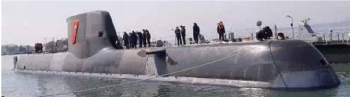
The lead submarine of the project, PIRI REIS , while floated in the water for the first time in Golcuk Shipyard. The flank array sonars are notable for being much longer than on the Type-214. Few other details are available however. Overall the current iteration of the MILDEN design appears a sensible design. It balances Turkey's desire to grow local industrial and technological capabilities with a design which is not too ambitious. MILDEN promises to take Turkish shipbuilding to the next level, joining the elite few which can design and build submarines. Source : NavalNews
