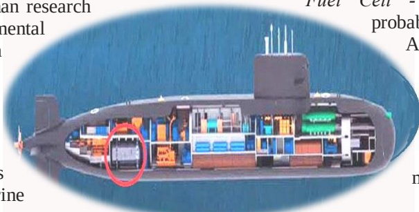
Illustration of the Chinese S-26 submarine, an oxygen tank for a Sterling cycle AIP system circled in red. China Shipbuilding Corporation Graphic
